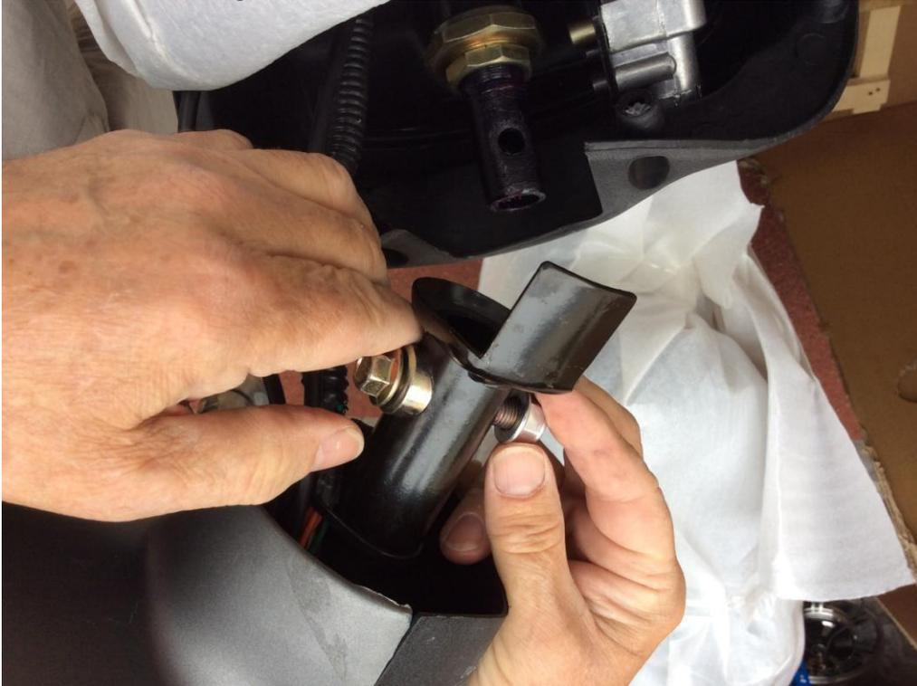
Turn the front wheel to the side to assist access. Slide the handlebars onto the stem and manipulate them until the bolt hole lines up. Put the bolt through the assembly and hand tighten with two 10mm spanners. Ensure that the handlebars are firmly secured and correctly at right angles to the front wheel. Turn to the full extent in each direction to ensure free movement.
