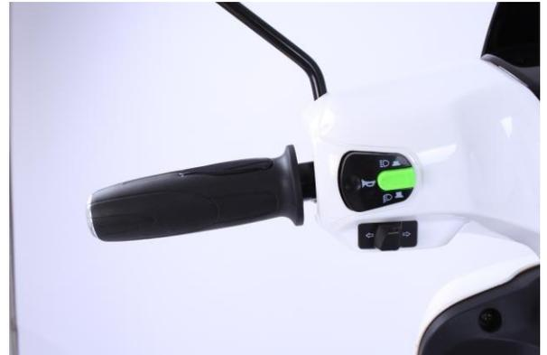
When riding downhill you must have the **E RIDER** switched on **even if you are not using the throttle** and even if the battery is not in the bike. Otherwise the motor will generate enough electricity to damage the controller beyond repair and this damage would not be covered by the warranty.
