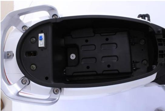
Turn the blue trip switch to the **off** position then unlock the battery panel with the ignition key and lift it up. Unplug the battery and remove it with the strap.
